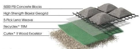
Flexamat<sup>®</sup> is a permanent erosion control mat . Also known as tied concrete block the blocks have a low profile (2.25") that fits the USACE, FEMA and FAA permitting. The 5,000 psi blocks (6.5" x 6.5") are embedded into a high strength geogrid, with a 1.5" spacing for Flexibility, Hydraulic relief, runoff absorption, and vegetated esthetics. With a low carbon foot print each truckload is equivalent to 33 truckloads of rock.
